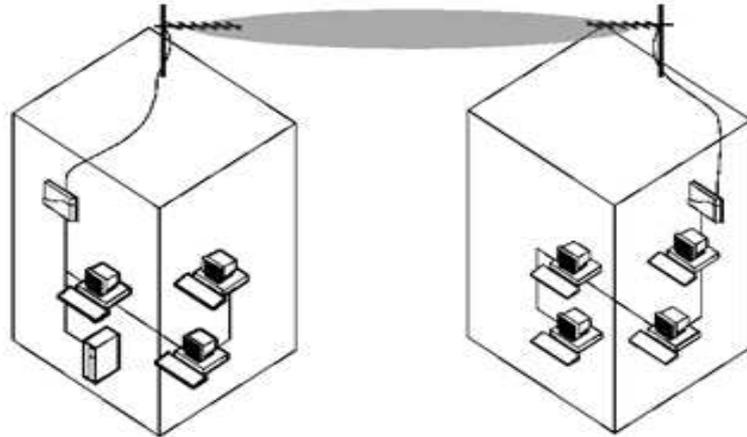
The Point-to-Point (PTP) Link functionality enables you to setup a connection
